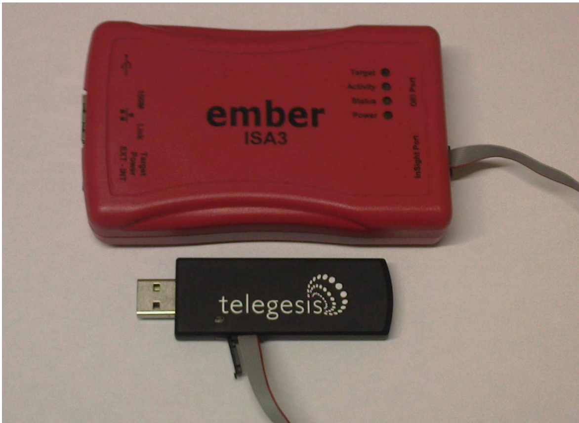
Figure 4: Connecting the ETRX357USB to the Ember ISA3
