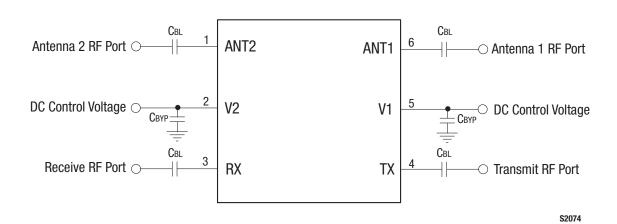
Figure 6. SKY13381-374LF Evaluation Board Schematic
