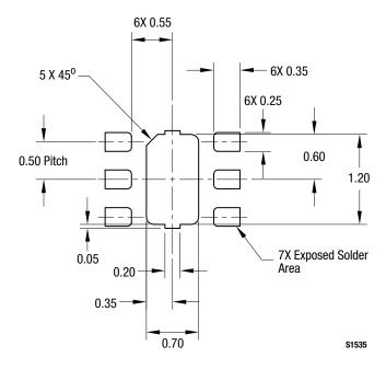
Figure 8. SKY13381-374LF PCB Layout Footprint (Top View)
