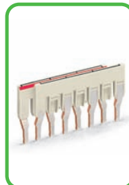
Two staggered jumpers 1 – 3 – 5 – 7 staggered for use in a jumper slot
