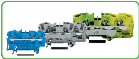
3-conductor terminal blocks 1.5 mm 2 (AWG 14); 2.5 mm 2 (AWG 12); 4 mm 2 (AWG 10); 6 mm 2 (AWG 8); 10 mm 2 (AWG 6); 16 mm 2 (AWG 4)
