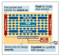
Instant-on (1ms), small-form-factor chip with support for high-speed 7:1 LVDS (840 Mbps) interface.
