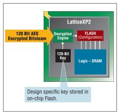
Design security ensured by a robust 128-bit AES bitstream encryption and design-specific key.
