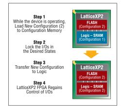
TransFR technology enables the LatticeXP2 FPGAs to be re-programmed while your system continues to operate.
