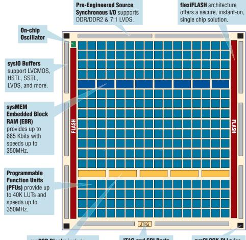
sysDSP Blocks include multiply and accumulate, up to 32 18x18 multipliers, and speeds up to 325MHz.
