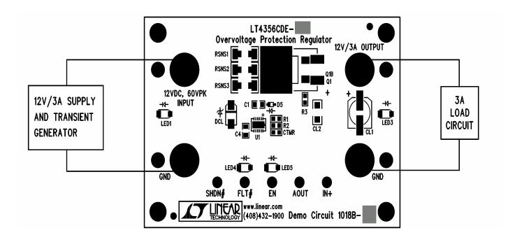
Figure 1: Proper Measurement Equipment Setup
