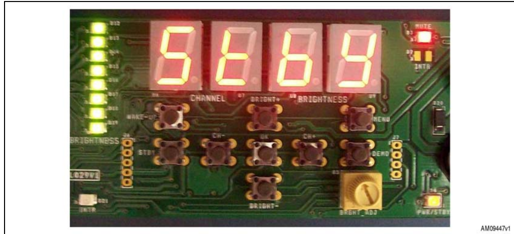
Figure 13. Entering into standby
