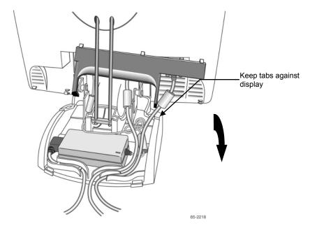
5. Lift this cover slightly so that the tabs are up against the rear of the display to keep them from catching on the cables below. Tilt the cover down as you slide the cover out from behind the support rods.
