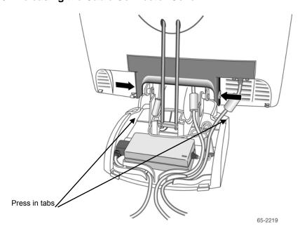
4. Push in on the cable connector tabs as shown above to release from display back. Gently pull down to release tabs.
