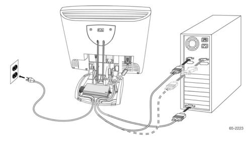
You should be sure all cable connections are secure -- tighten all cable screws. Shaking and vibration may dislodge cables that are improperly connected.
