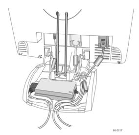
Figure 6. Disassembling the Display from Its Base for Arm Mounting
