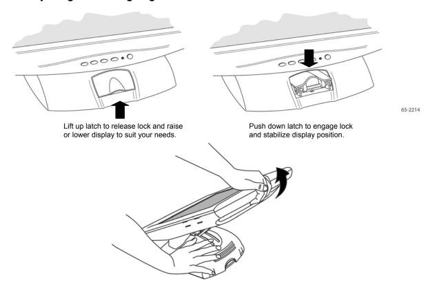
Lift up on the latch to release lock. Adjust the M1700SS Display by pushing or pulling on the top front of the display until the screen is at the best viewing angle for you. Then push down on latch to engage locking mechanism and stabilize display position.
