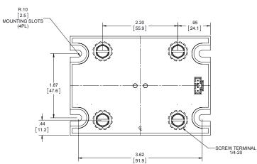
Tolerances:  $\pm\,0.02$  in / 0.5 mm. All dimensions are in: inches [millimeters]
