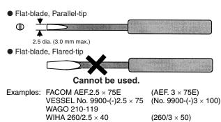
\*Chamfering the tip of the driver improves insertion when used as an exclusive tool.
