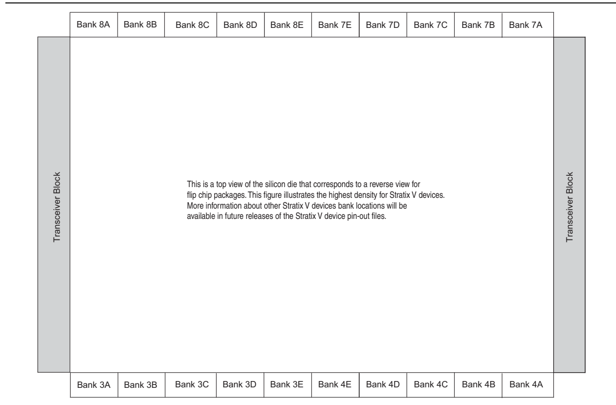
Figure 5-1. I/O Banks for Stratix V Devices—Preliminary
