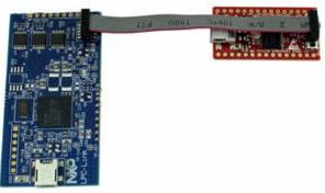
Use a debugger and JTAG adapter of your choice which supports the Cortex-M3 ARM core and more specifically the NXP LPC1343 microcontroller. You might need an adapter such as the <u>10-pin to 20-pin JTAG Adpater Kit</u> between your JTAG solution and the target board.
