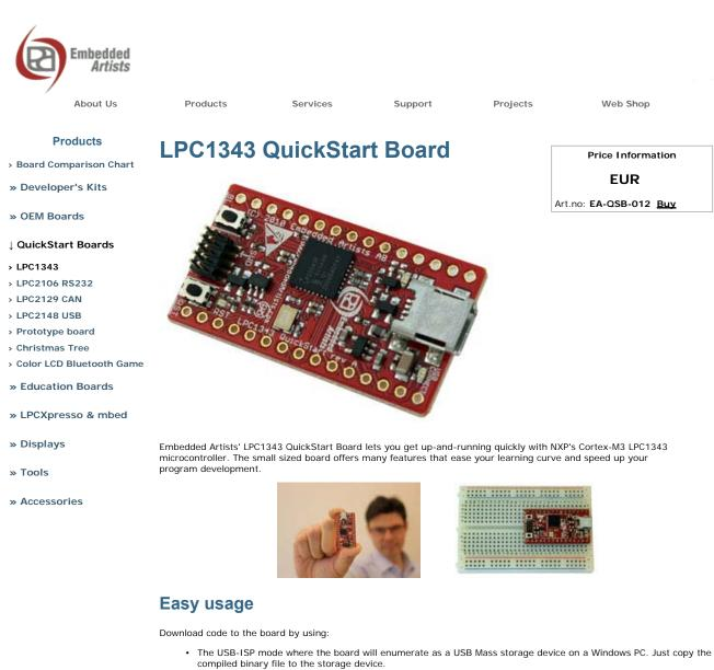
Use the free <u>LPCXpresso IDE/Debugger</u> together with, for example, an LPC-Link, a <u>10-pos IDC Ribbon cable</u> and connect to the SWD interface (10-pin JTAG connector) on the board, see figure below. This allows you to both download and debug code on the board.
