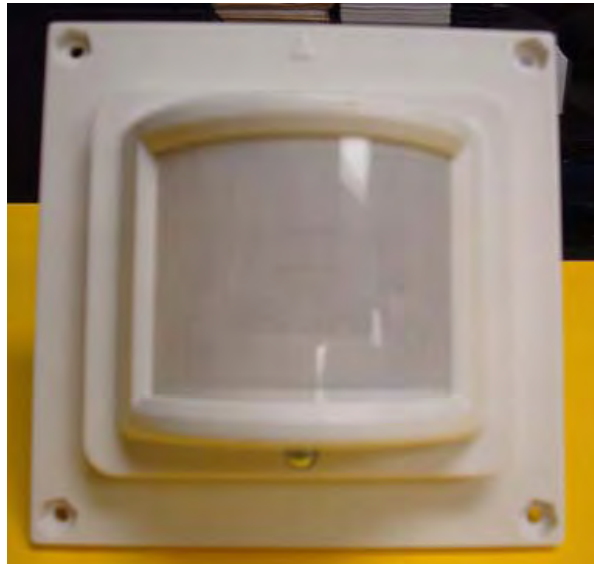
Figure 5. Assembled Flat 1.2" Lens Holder and Flat Lens
