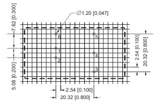
Pin section tolerances:  $\pm 0.10mm[\pm 0.004inch]$ General tolerances:  $\pm 0.25mm[\pm 0.010inch]$
