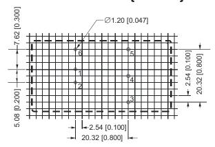
Pin section tolerances:±0.10mm[±0.004inch] General tolerances:±0.25mm[±0.010inch]
