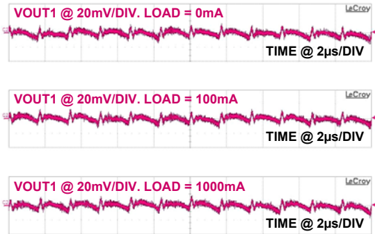
FIGURE 23. PWM1 OUTPUT RIPPLE, MODE = 5V (CCM)
