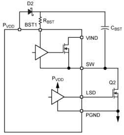
Figure 5. High-side Drive Circuitry
