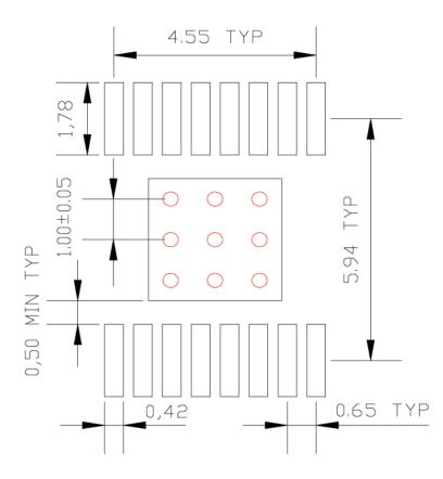
Red circle indicates Thermal Via. Size should be .300-.350 mm in diameter and it should be connected to GND plane for maximum thermal performance.
