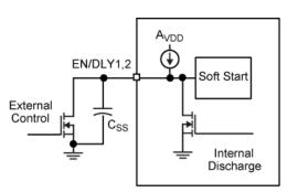
Figure 1. Enable and soft-start circuit
