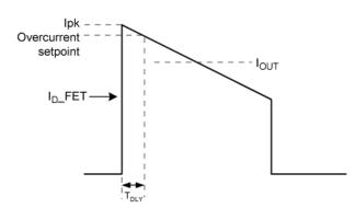
Figure 9. Overcurrent waveform
