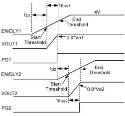
Figure 4. Output Sequencing Waveforms
