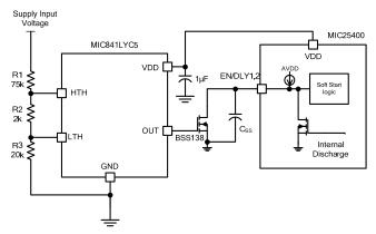
Figure 1A. Adjustable UVLO startup circuit
