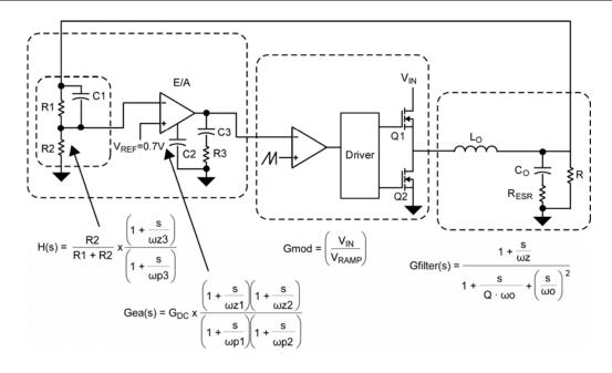
Figure 12. Voltage Loop and Transfer Functions
