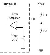
Figure 8. Setting the Output Voltage
