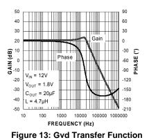
If the output capacitance and/or ESR is high, the zero moves lower in frequency and helps to boost the phase, leading to a more stable system.
