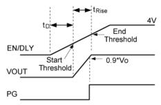
Figure 2. Soft-start Timing Diagram
