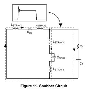
Proper snubber design requires the parasitic inductance and capacitance be known. A method of determining these values and calculating the damping resistor value is outlined below.
