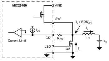
Figure 7. Over-current Circuit
