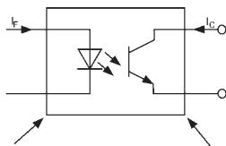
One important variable of this component is the current transfer rate (CTR). The CTR factor is stated as a percentage and describes the ratio between dispensed input current  $I_F$  and the maximum available output current  $I_C$ .
