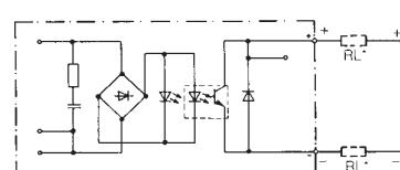
Here it is not possible to reverse the polarity of the DC input signal. The disadvantage of the AC/DC input circuit
