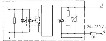
A special semiconductor module (TRIAC) is used for switching AC voltage in the output stage of the optocoupler. Here, as with the DC output, consideration must also be given to the key data such as voltage, frequency, maximum load current and ambient temperature.
