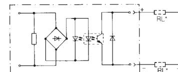
Here again, the charging capacity has a major influence on the maximum switching frequency of the module as a whole. Weidmüller optocouplers with AC/DC or AC input signals are rated for mains frequencies of approx. 40 – 60 Hz. In the case of AC input signals, the maximum switching frequency of the optocoupler module is less than half the mains frequency. A higher switching frequency is not possible, because this would result in constant switching in the rhythm of the mains frequency.
