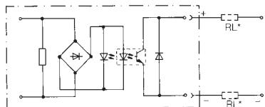
The 2-pole DC output can be compared with a conventional switch. In this version it does not matter where the load is located (in the output circuit), although the necessary output supply voltage must be available with the right polarity.
