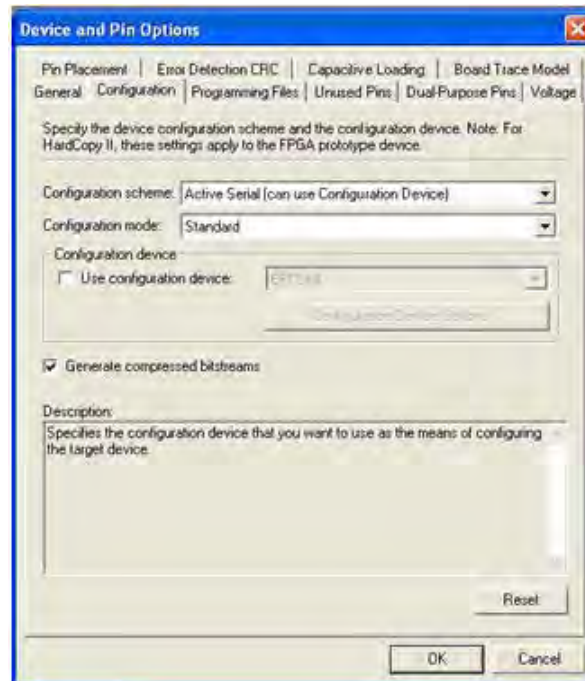
Figure 10-19. Enabling Compression for Stratix IV Bitstreams in Compiler Settings
