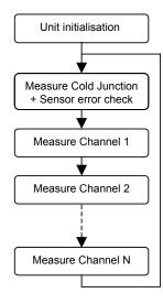
The cold junction compensation measurement and one sensor error check are executed each cycle.
