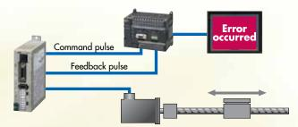
Simplified Synchronization: It is also possible to input encoder output signals directly into the servo drive.
