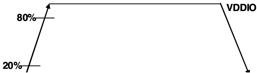
Figure 4. Output Pad Transition Waveform
