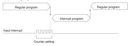
There are two quick-response inputs for the CPM1A 10-point I/O CPU and four for the 20-, 30-, and 40-point I/O CPU (shared with the interrupt inputs). Since an internal buffer is provided, the quick-response input function can even detect signals modified within one cycle.
