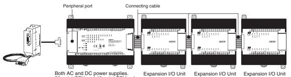
Both AC and DC power supplies. Expans 30-point CPU and 40-point CPU only. May be expanded up to a maximum of 3 Units.
