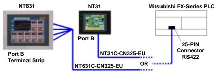
The FX0 and FX0N PLCs use a different connector than the other FX series PLCs. Connect the Omron cable to the FX-20P-CADP cable from Mitsubishi, then connect it to the PLC communication port.
