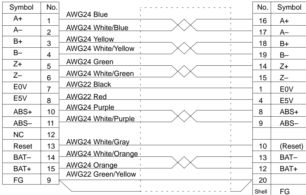
Cable: AWG22 × 3C + AWG24 × 6P
