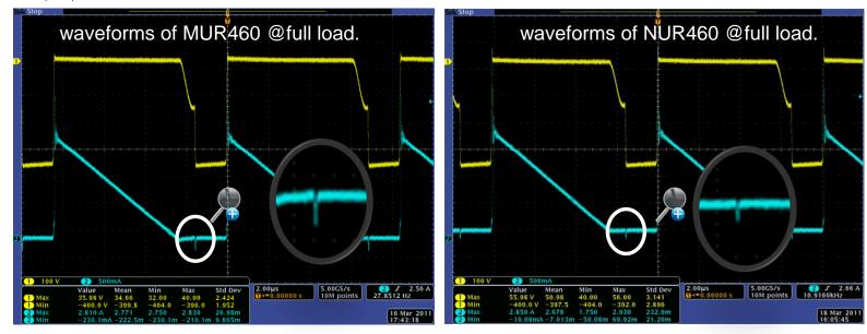
The blip in the highlighted area shows the reverse recovery current of D1 at the moment when the voltage on it rises rapidly. At this point the MOSFET voltage is still significant, and the blip in the diode current appears as an additional turn-transient in the MOSFET. Needless to say, the smaller blip of NUR460 leads to less heat dissipated into MOSFET.
