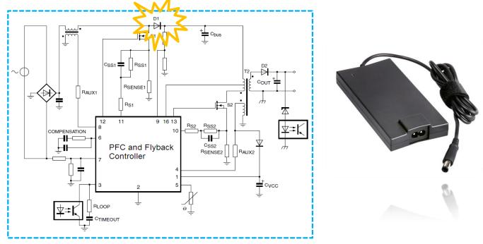
The PFC block create a 380V ~ 400V (DC) supply voltage using a high performance axial leaded NUR460 designated D1 in the circuit diagram.
