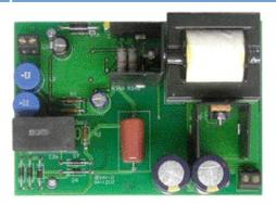
output) PFC converter as demonstrated in this evaluation circuit, which is designed for a 48 Vdc, at 1.9 A of output current. The NCP1651 is designed to operate in the fixed frequency, continuous mode (CCM), or discontinuous mode (DCM) of operation, in a Flyback converter topology.
