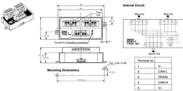
**Note:** When connecting a branch line to the main line, connect the main line to the connector marked with an asterisk because the resistance between the asterisked portion is minimal.
