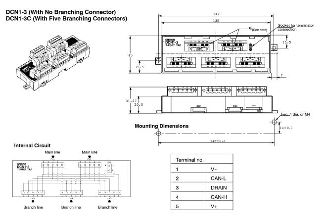
**Note:** When connecting a branch line to the main line, connect the main line to the connector marked with an asterisk because the resistance between the asterisked portion is minimal.
