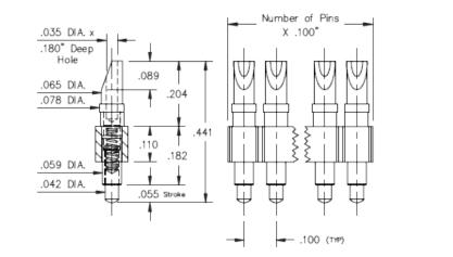
**Description:** Interconnect Header Spring-Loaded Header Soldercup Tail Single Row Plating Code: 22
