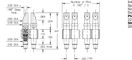
**Description:** Interconnect Header Spring-Loaded Header Soldercup Tail Double Row **Plating Code:**
