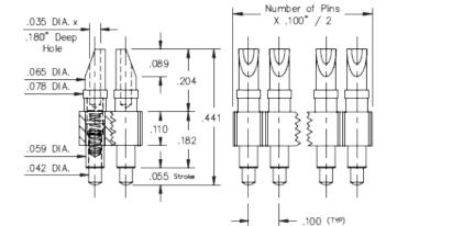
**Description:** Interconnect Header Spring-Loaded Header Soldercup Tail Double Row **Plating Code:** 22
