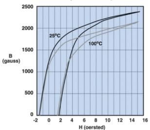
Measured on a 19/10/6mm toroid at 10kHz.
