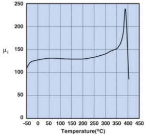
Measured on a 19/10/6mm toroid at 100kHz.
