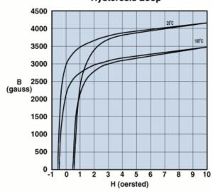
Measured on a 17/10/6mm toroid at 10kHz.
