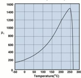
Measured on a 17/10/6mm toroid at 100kHz.
