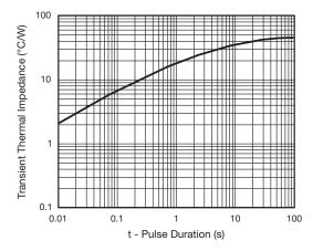
Fig. 6 - Typical Transient Thermal Impedance
