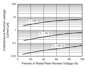
Fig. 4 - Typical Reverse Characteristics
