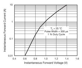
Fig. 3 - Typical Instantaneous Forward Characteristics
