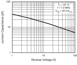
Fig. 5 - Typical Junction Capacitance
