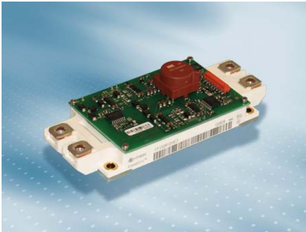
Figure 1 The 2ED100E12-F2 Evaluation Driver Board mounted on the top of the EconoDUAL™3 module
