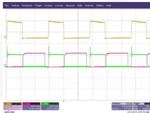
Figure 7. FAN6754AMR+FAN6204MY, 115V/60Hz, 80% Load (Ch1: Gate, Ch2: Gate_SR, Ch4: V dS )
