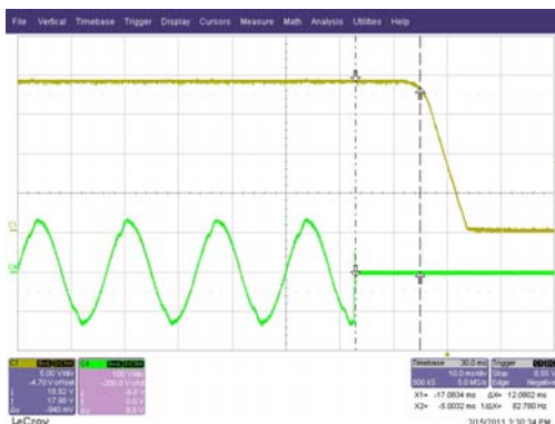
Figure 16. 90V / 60Hz at Maximum Load (Ch1: V OUT ; Ch4: V AC )
