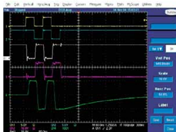
Fig 2: INA, INB, OUTA, OUTB and HV OUT with 220pF//1K Load, V DD = V H = +12V, V SS = V L = 0V, V PP /V NN = +/-100V, 20MHz
