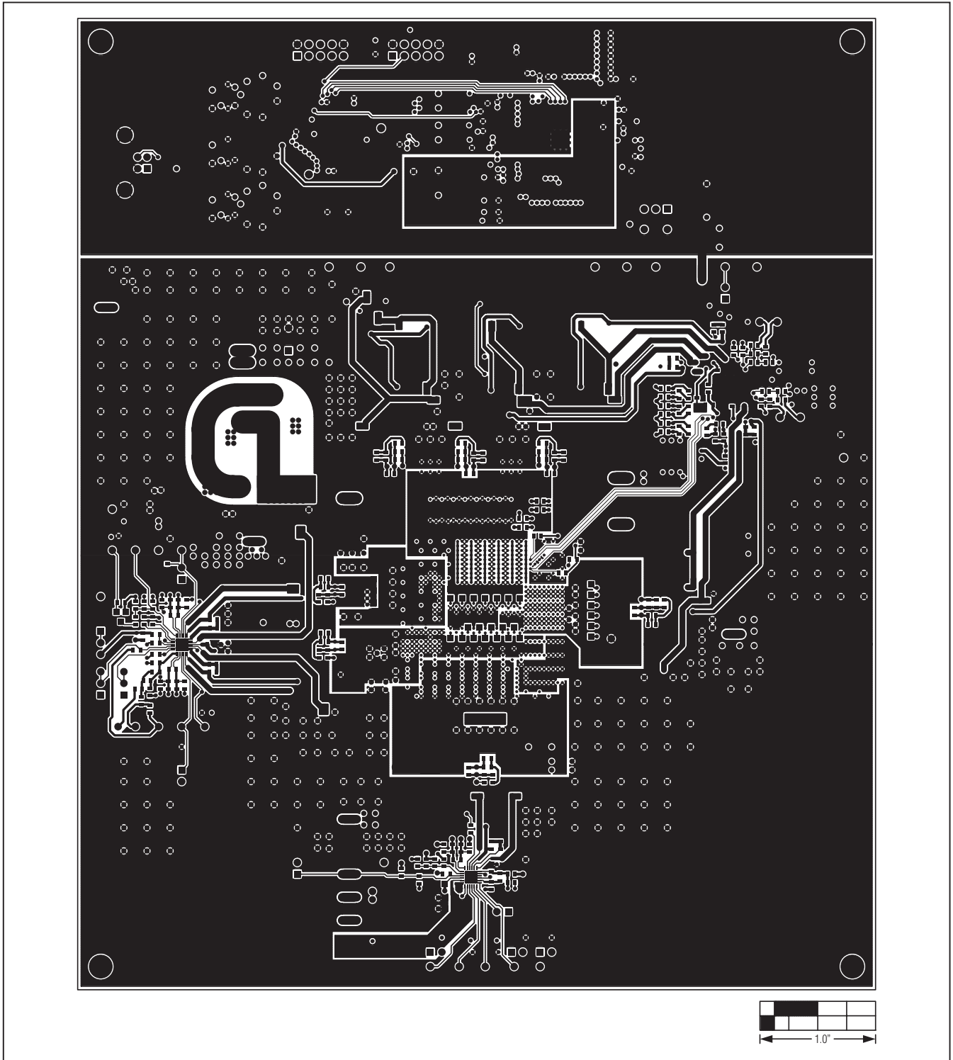
Figure 14. MAX17039 EV Kit PCB Layout—Solder Side
