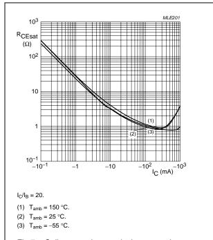
Fig.7 Collector-emitter equivalent on-resistance as a function of collector current; typical
