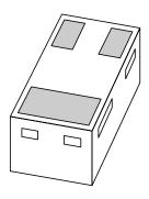
PBSS3540M 40 V, 0.5 A PNP low V<sub>CEsat</sub> (BISS) transistor
