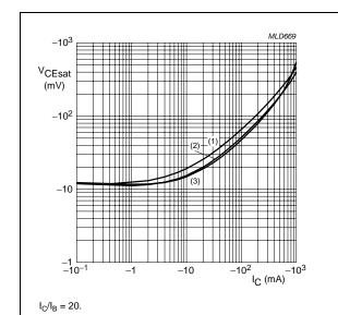
(1)  $T_{amb} = 150 \,^{\circ}\text{C}$ . (2)  $T_{amb} = 25 \,^{\circ}\text{C}$ .
