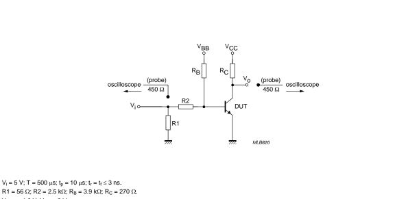
Fig.7 Test circuit for switching times.
