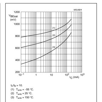
Fig.5 Base-emitter saturation voltage as a function of collector current.
