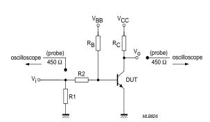
$$\begin{split} &V_i = 9.5 \; V; \, T = 500 \; \mu s; \, t_p = 10 \; \mu s; \, t_r = t_f \leq 3 \; ns. \\ &R1 = 68 \; \Omega; \; R2 = 325 \; \Omega; \; R_B = 325 \; \Omega; \; R_C = 160 \; \Omega. \\ &V_{BB} = -3.5 \; V; \; V_{CC} = 29.5 \; V. \\ &Oscilloscope input impedance \; Z_i = 50 \; \Omega. \end{split}$$
