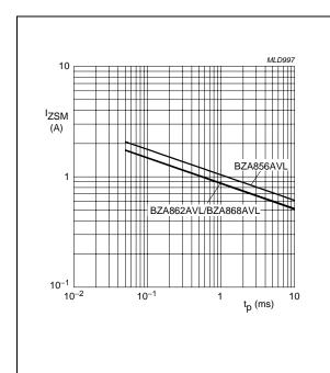
Fig.2 Maximum non-repetitive peak reverse current as a function of pulse time.
