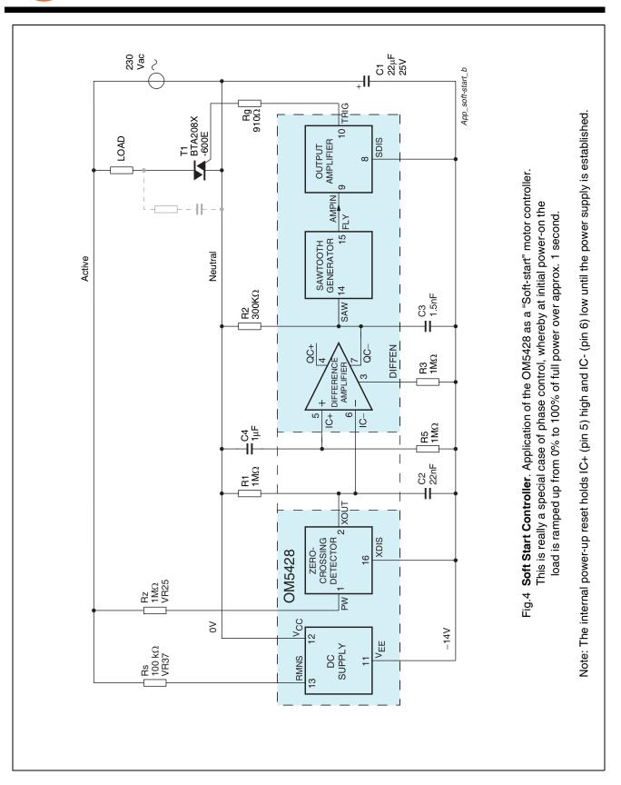
Hendon semiconductors Phase Controller and Triac Triggering IC
