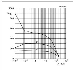
**BC857B**;  $V_{CE} = -5 \text{ V}$ .
