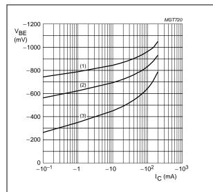
**BC857C**;  $V_{CE} = -5 \text{ V}.$
