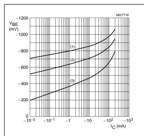
**BC857B**;  $V_{CE} = -5 \text{ V}.$
