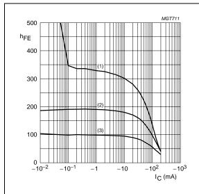
**BC857A**;  $V_{CE} = -5 \text{ V}$ .
