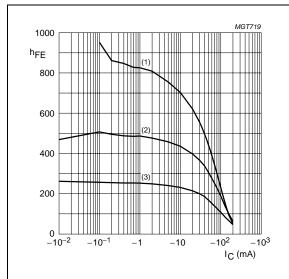
**BC857C**;  $V_{CE} = -5 \text{ V}.$
