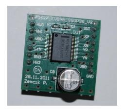
For the test of this DUT, the ON semiconductor evaluation kit for the AMIS\_306xx and ON Semi\_30627 has to be used. The procedure assumes that the test engineer is familiar with the use of the evaluation board and the GUI software.
