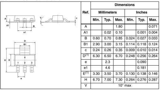
1. Do not include mold flash or protrusions. Mold flash or protrusions shall not exceed 0.15mm (0.006inches)
