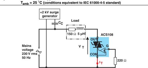
Figure 18. Overvoltage ruggedness test circuit for resistive and inductive loads,
