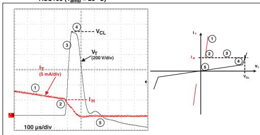
Figure 17. Switching off of a high inductive load - typical clamping capability of ACS108 ( $T_{amb}$  = 25 °C)
