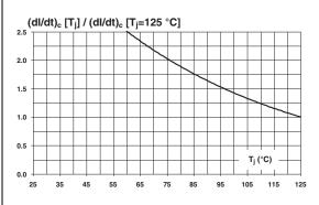
Figure 12. Relative variation of static dV/dt immunity versus junction temperature<sup>(1)</sup>
