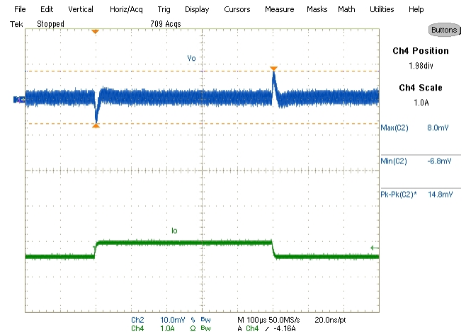
Transient response-Sinking mode Vin-1.5V Vout-0.75V/3.9-4.3-3.9A Ch4-Vout Ch3-Iout (1A/µSec slew rate)
