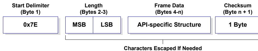
Figure 6-02. UART Data Frame Structure - with escape control characters:
