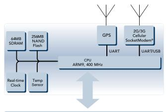
80 pin B2B connector Battery / GPIO / ADC / SPI / I2C / JTAG / Ethernet / USB Host / USB Device / GPS PPS - Data / Serial UARTs / LEDs
