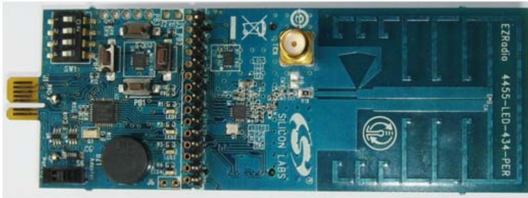
Figure 1. Si4455 RFStick 434 MHz Transceiver Board (P/N 4455-LED-434-PER)
